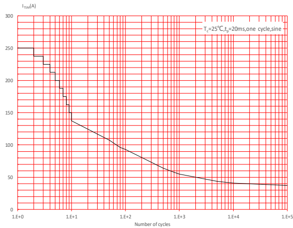
FIG.5: Non-repetitive surge peak on-state current for a sinusoidal pulse with width t_p < 20\text{ms} , and corresponding value of I^2t ( di/dt < 100\text{A}/\mu\text{s} )
